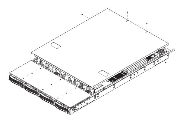
Figure 2-4. Accessing the Inside of the System
